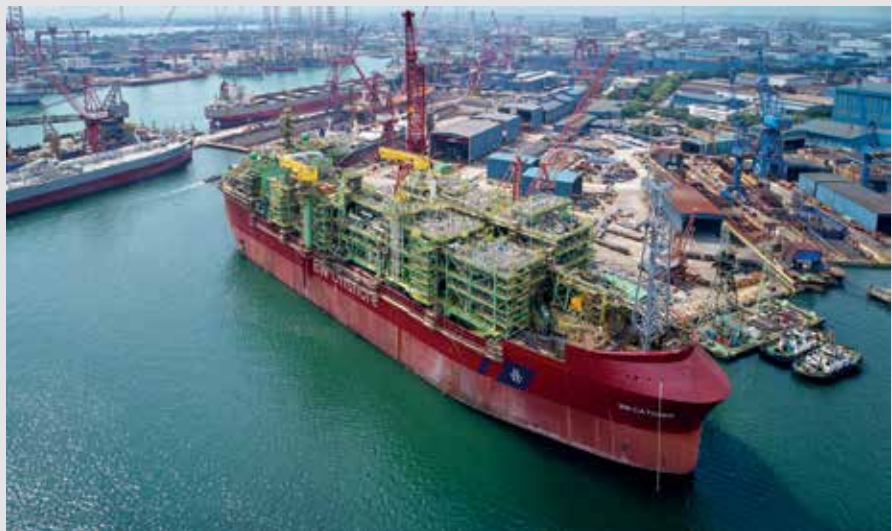
Delivered in the third quarter of 2017, the FPSO BW Catcher has an oil storage capacity of 650,000 barrels, with a processing capacity of 60,000 barrels per day
