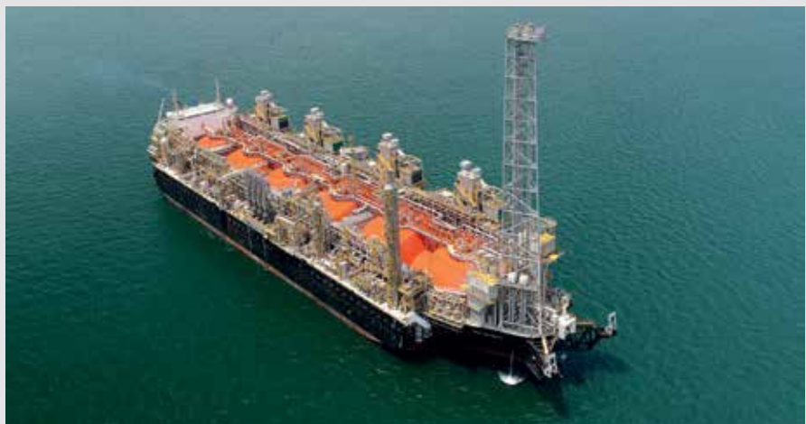
Hilli Episeyo, the world's first FLNG conversion project, was converted from a 1975-built Moss LNG carrier with a storage capacity of 125,000 m 3
